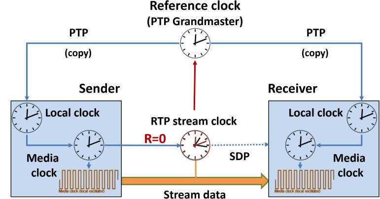
The offset (R) will be conveyed via SDP (a=mediaclk:direct=<offset>) - must be "0" in ST2110
