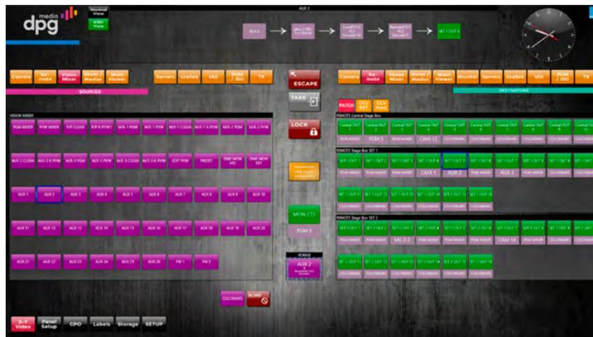
VSM software panel of the "Engineering View" in the top row: all C100 blades involved in a process are shown in the correct sequence.
