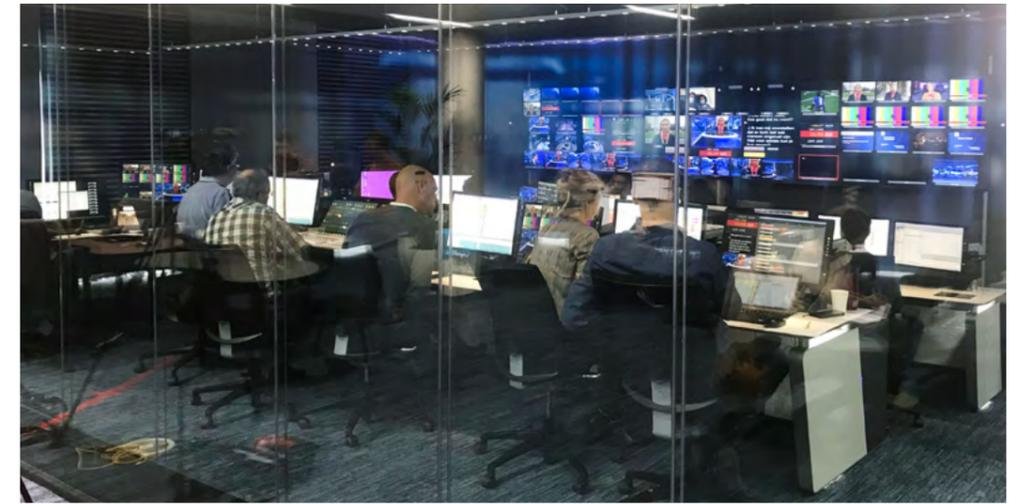
Much smaller than the two control rooms in Vilvoorde, the **production gallery in Antwerp** is equipped with a compact, dual-fader **mc<sup>2</sup> 56** audio production console. It is located in the same room that also houses the video gear.
