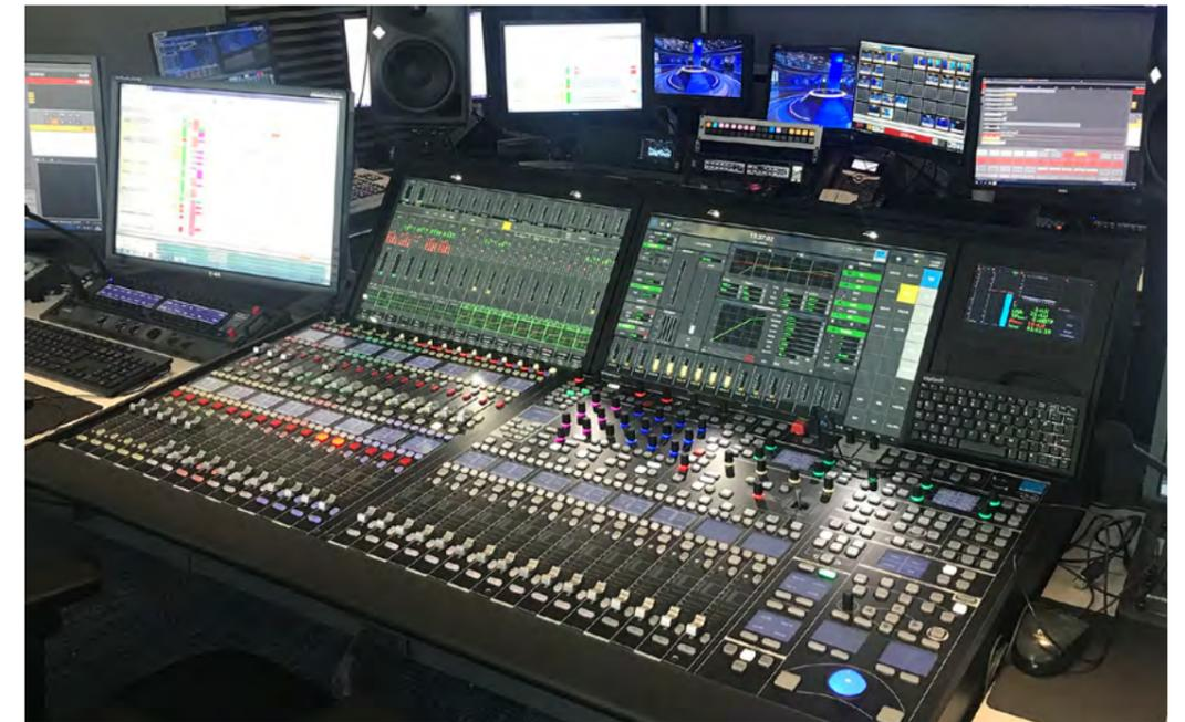
mc<sup>2</sup>56 Audio Production Console in Antwerp. It has access to 256 DSP channels of an A\_\_UHD Core unit in Vilvoorde.
